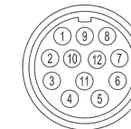
HA connector (12 pin) - M23 CCW Hummel 7.410.000000 - 7.002.912.603 front view
