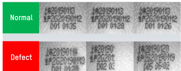
Food packaging character defect detection: using deep learning algorithms to achieve defect detection of spray code characters on food packaging.
