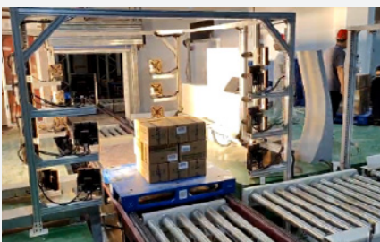
Enterprise warehousing corridor code reading
