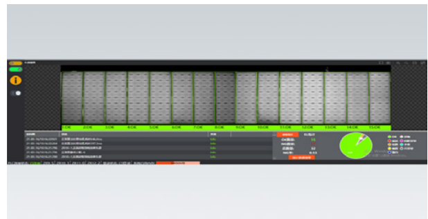
PV panel defect detection: using deep learning with traditional algorithms for defect detection during EL inspection of PV panels.
