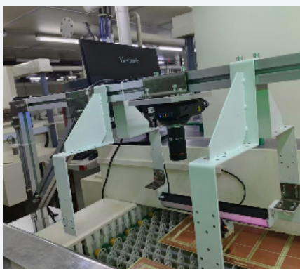
Covered PCB code reading
